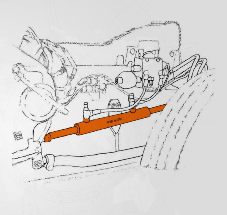
The primary function of the **Steering Cylinder** is to provide hydraulic power assistance to the steering system of commercial vehicles. It works in conjunction with the main power steering system and helps reduce the effort required to steer the vehicle, especially at low speeds and during maneuvers. By utilizing hydraulic pressure, the cylinder amplifies the driver's input, allowing for more controlled and effortless steering.
