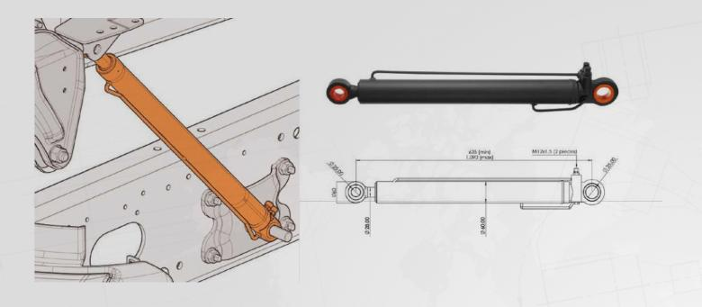
The **Cabin Tilting Cylinder**, also known as the **Cab Tilt Cylinder**, is an essential component used in commercial vehicles, particularly trucks, to facilitate the tilting of the **driver's cabin** towards the front. This feature **enables easy and safe** access to the engine compartment, allowing for efficient maintenance and servicing.
