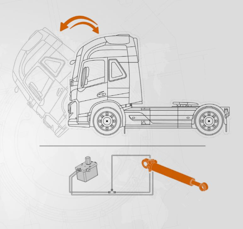
The primary function of the Cabin Tilting Cylinder is to generate hydraulic force that enables the controlled tilting motion of the driver's cabin. It operates by utilizing hydraulic pressure to extend and retract a piston, which in turn moves the tilting mechanism. The cylinder is usually integrated with a locking system that securely holds the cabin in position during maintenance operations.
